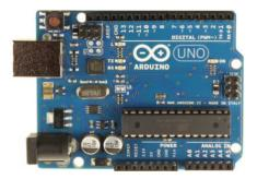
Arduino is an open-source electronics prototyping platform based on flexible, easy-to-use hardware and software. It's intended for artists, designers, hobbyists and anyone interested in creating interactive objects or environments.
