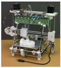
References: http://reprap.org/wiki/RepRap RepRap was the first of the lowcost 3D printers, and the RepRap Project started the open-source 3D printer revolution.
