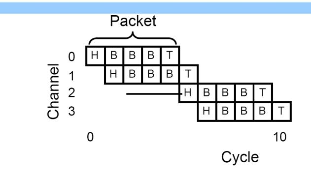
Transmission on the next channel starts directly when the new header flit is received (otherwise it behaves like Store-Forward)
