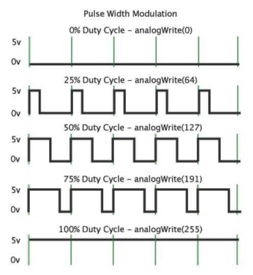
In this graphic, the green lines represent a regular time period. This duration or period is the inverse of the PWM frequency. In other words, with Arduino's PWM frequency at about 500Hz, the green lines would measure 2 milliseconds each.
